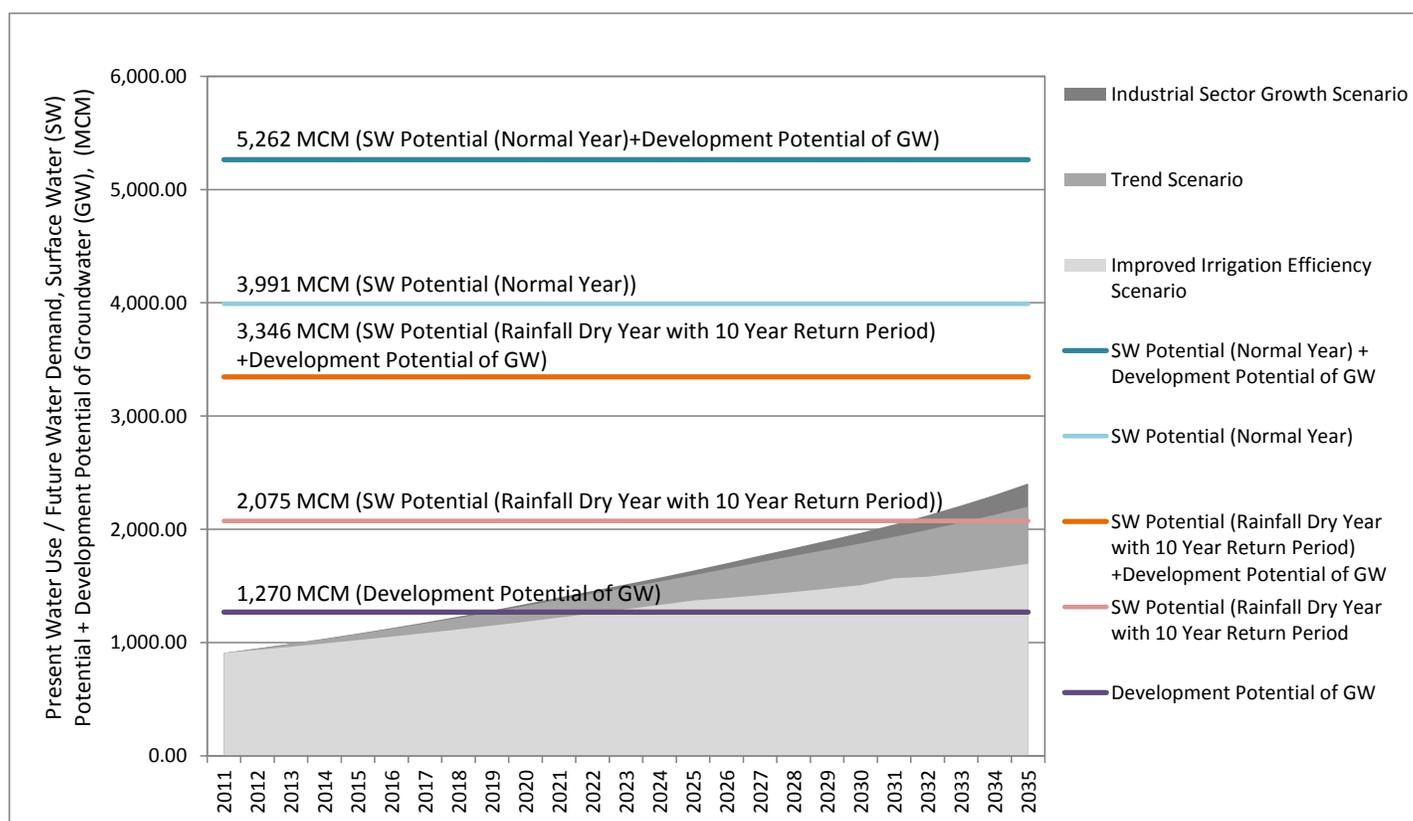
Figure 4-4: Water demand of three scenarios (trend, improved irrigation, and industrial growth) and water resources availability (surface water potential and development potential of groundwater) in the Wami/Ruvu Basin. [Source: JICA 2013]
