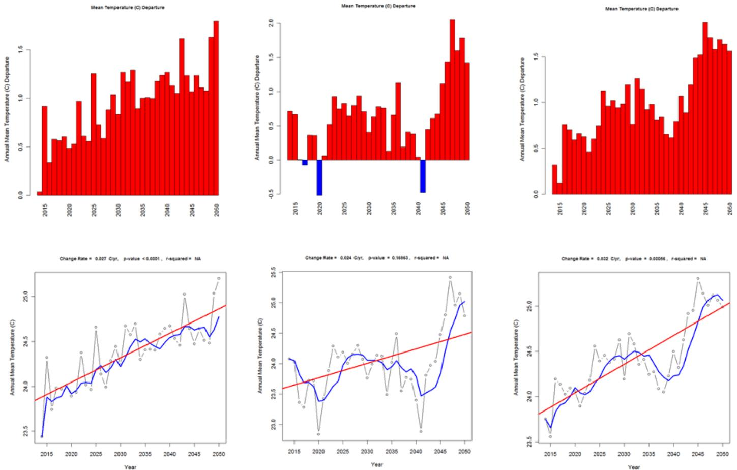
Figure 2-27: (Upper panel) Yearly mean temperature (2014-2050) deviations from the 1961-1990 mean by MIROC3.2 (left), CSIRO-Mk3.0 (middle) and UKMO\_had3.1 (right) models under A2 emission scenario. Bars in red indicate an increase in annual mean temperature while blue bars indicate a decrease. (Lower panel) Yearly mean temperature predictions by the three models. [Data Source: ClimateWizard]
