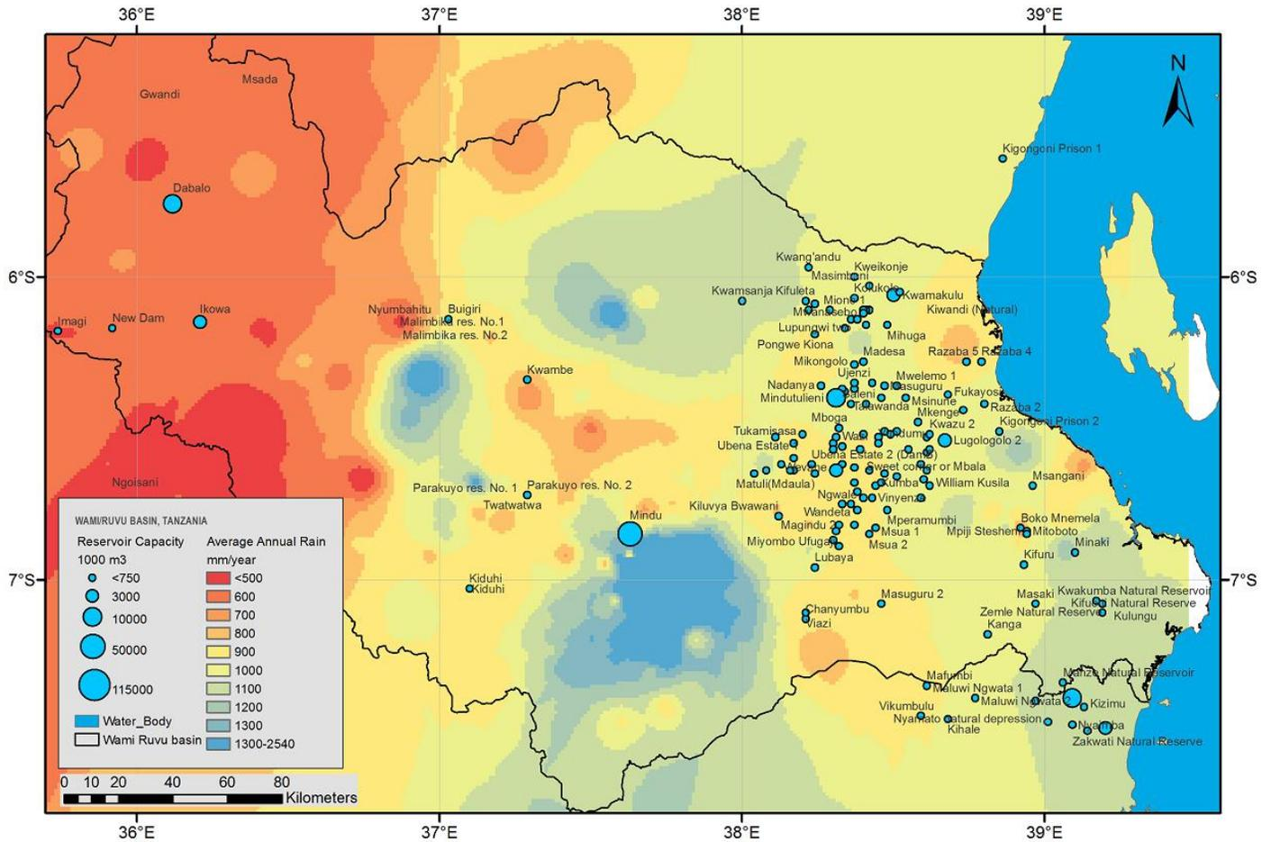
Figure 5-1: Surface water reservoirs existing in the Wami/Ruvu Basin over a backdrop of the average annual rainfall. [Data: WRWBO]
