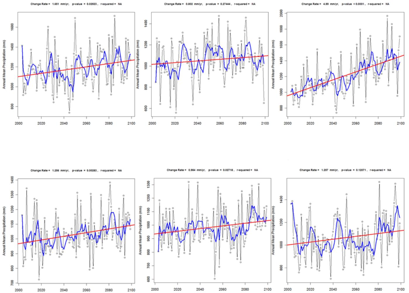
Figure 0-3: annual precipitation projections (2000-2099) by models inmcm3\_0.1, giss\_model\_er.1, micro\_3\_2Medres, miub\_echo\_g.1, mpi\_echam5.1 and ipsl\_cm4.1. [Data Source: ClimateWizard]
