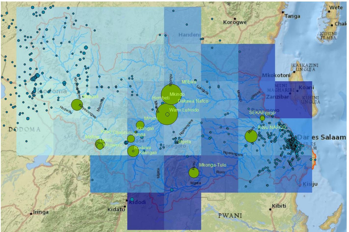
Figure 4-7: Location of borewells (blue circles) and irrigation projects (green circles) in the Wami/Ruvu Basin (orange boundary) overlaid over the mean Annual Precipitation (mm) at a 50 km grid scale. Circle size reflects relative amount of groundwater extraction for borewells and surface water use for irrigation. [Data Source: ClimateWizard and WRBWO]
