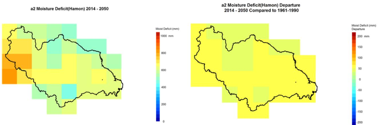
Figure 2-38: (Left) Soil moisture deficit predicted by an ensemble of 16 GCMs at A2 scenario as an average over 2014-2050. (Right) difference between predicted soil moisture deficit and the average soil moisture deficit prevailing over 1961-1990. [Data Source: ClimateWizard]
