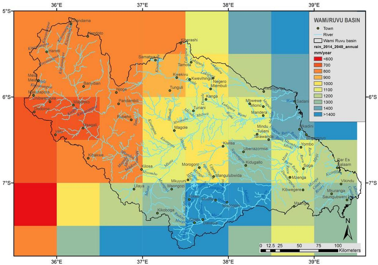
**Figure 2-28: Predicted average annual precipitation (2014-2040) by an ensemble of 16 GCMs at A2 emission scenario for the Wami/Ruvu Basin. [Data Source: ClimateWizard]**
