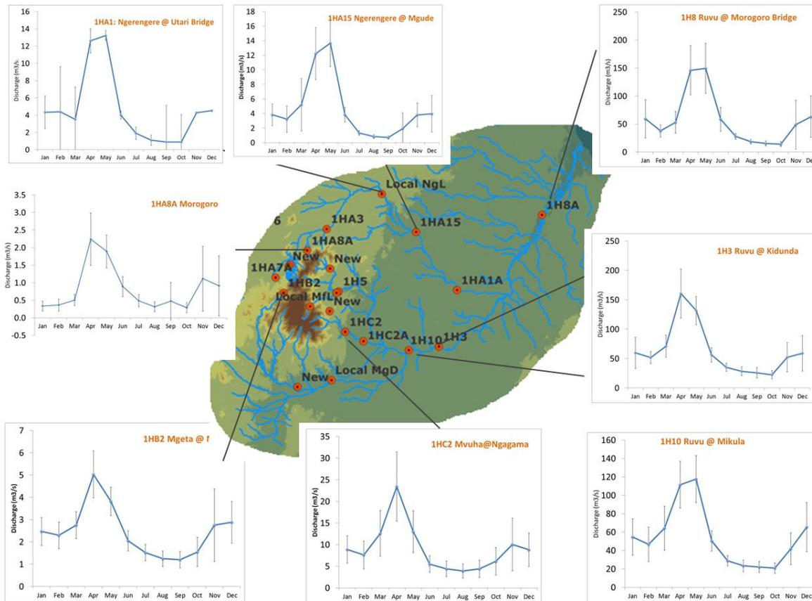
Figure 4-5: Monthly discharge (1952-2010) in the Ruvu Basin. Error bars represent standard deviation for each month, portrayed as half above and half below the mean for display purposes. [Data Source: WRBWO]
