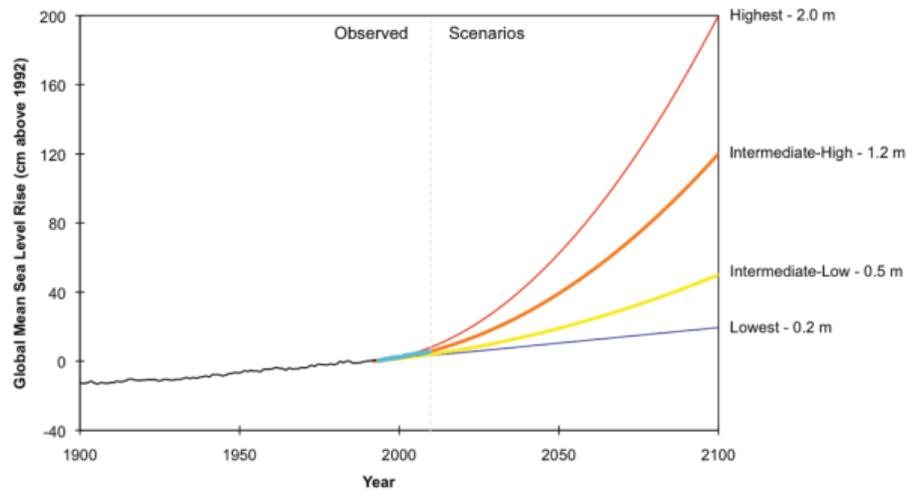
Figure 2-18: Global average SLR from the 1900s and projected SLR. [Source: Parris *et al.* 2012]
