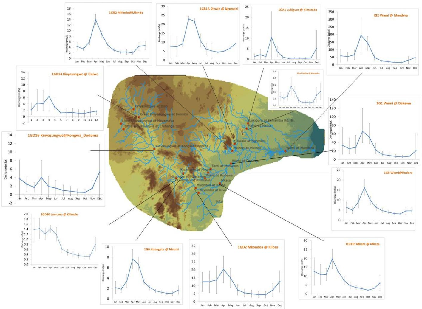
Figure 4-6: Monthly discharge (1952-2010) in the Wami Basin. Error bars represent standard deviation for each month, portrayed as half above and half below the mean for display purposes. [Data Source: WRBWO]
